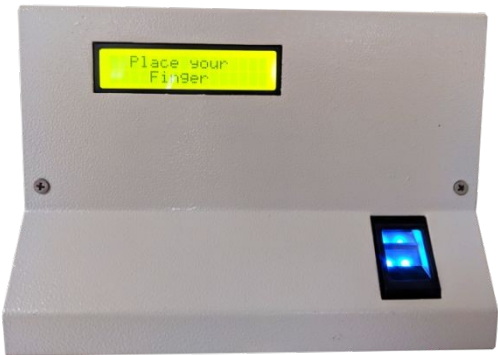
ACCESS CONTROL SYSTEM
