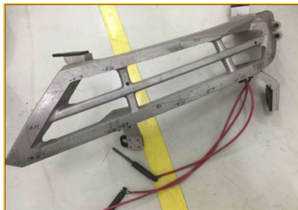
Car Headlights mounting dimension verification Jig
