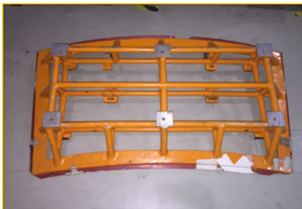
Car Windshield mounting dimension verification Jig
