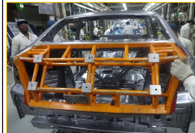
Trunk lid mounting dimension verification Jig
